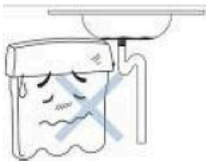
If it is used while the sewer is blocked, it may cause the waste water to back up or pollution to get inside the water purifier.
