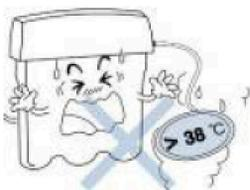
If the inlet water temperature is over 38°C, it will damage the reverse osmosis membrane leading to membrane failure.
