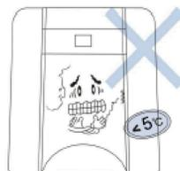
If the temperature in the room is below 5°C, please be sure to take measures to prevent freezing, such as starting the heater or air conditioner to prevent leakage or cracked pipes caused from water freezing inside the machine
